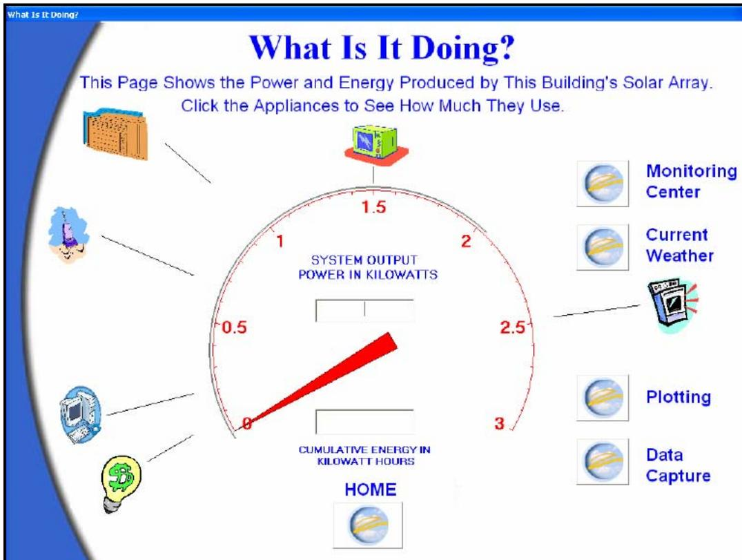
The focus of this page is the power meter. This meter shows how many kilowatts of power are being produced at any given time. In the center of the meter you can see the numerical readout for the meter. At the bottom of the meter is a numerical readout showing how many kilowatt-hours of energy have been produced since the system was installed.
