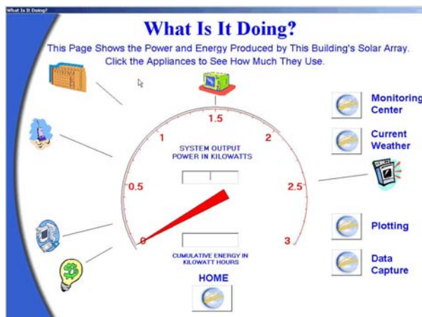
Figure 18. Meters on the graphical interface at each school move in real time as the inputs change. The “speedometer” and “odometer” illustrate 1) that meters can have more than one application and 2) how speed and distance have the same mathematical relationship as power and energy – a concept that can be taught quantitatively, (cut out the area under the curve and weigh it) algebraically, or with calculus.
